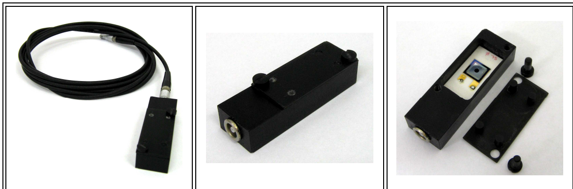
Figure 2. Photographs of the plastic container for diode MCz.
