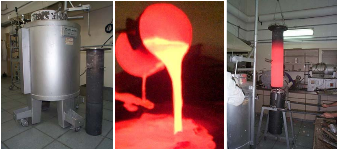
Figure 4: Heating system and reactor vessel (left), molten salt (center), reactor with molten salt removed from the heating system.
