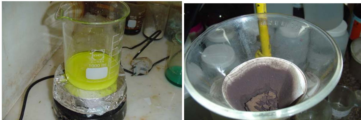
Figure 5: Dissolution of the salt and filtering to separate the present oxides.
