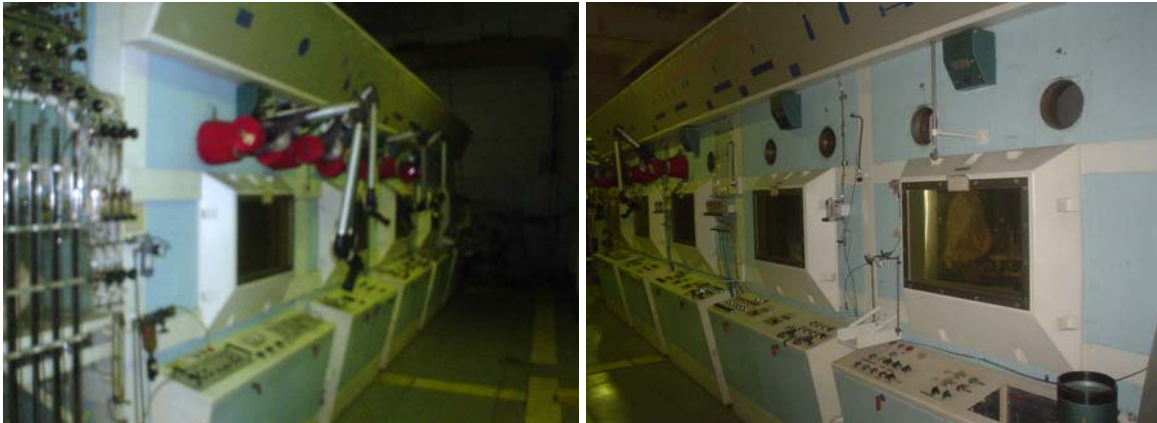
Figure 1: Hot cells of the CELESTE-1 laboratory.
