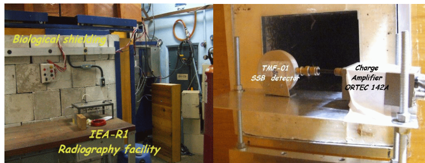
Figure 3. Neutronography assembly (left) and the TMF-1 SSB Detector setup (right).
