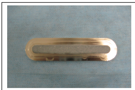
Figure 1. Electroplated Zn Target in Cu/Ni plates
