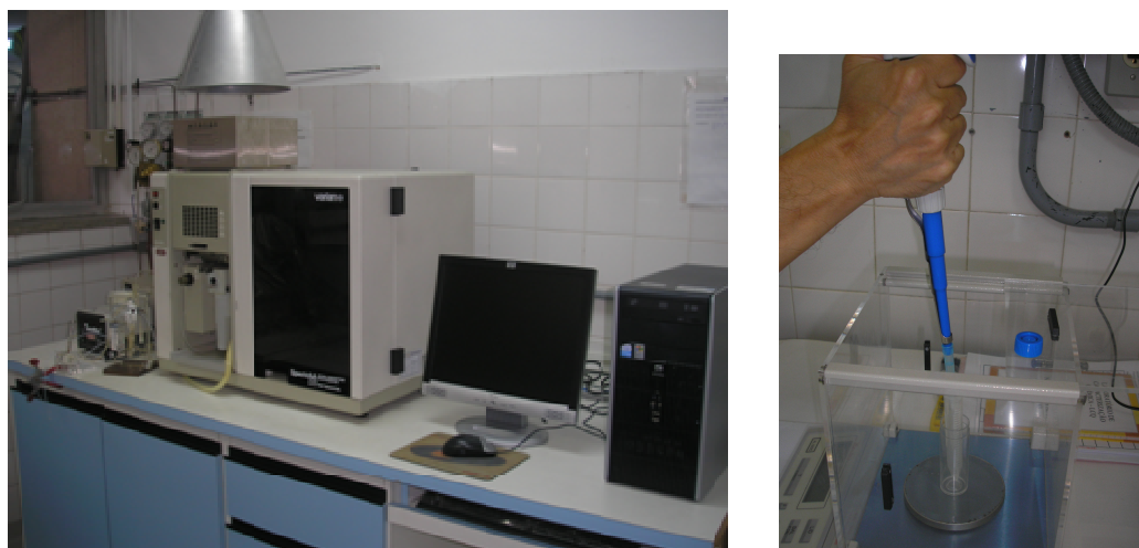
Figure 2. Atomic absorption spectrometer Spectra AA-220 Fast Sequential and standard gravimetric preparation.
