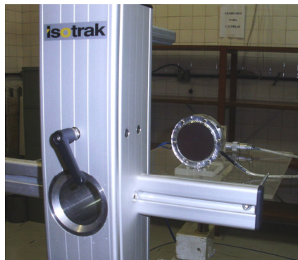
Fig. 6. Parallel plate ionization chamber positioned at the BSS2 system during the calibration procedure.
