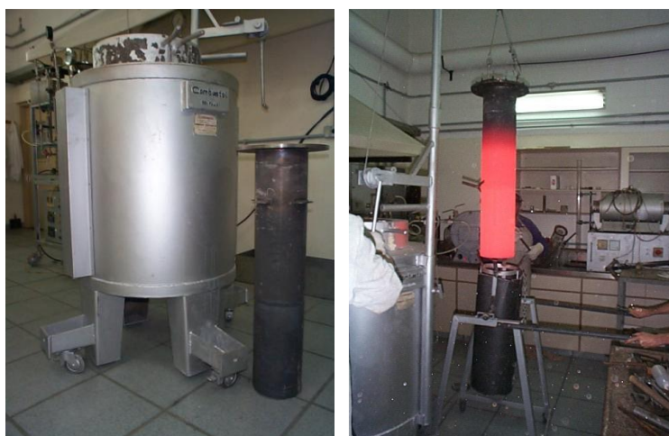
Figure 4: Heating system and reactor (left), hot reactor removed from the heating system (right).
