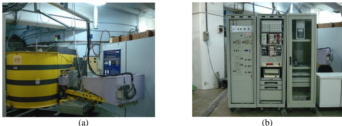
FIG.1. The HRPD Aurora (a) and the three racks with the associated electronics and control modules used in control and data acquisition (b).
