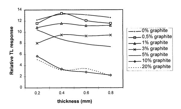
Figure 1: Relative TL response as a function of pellet thickness and graphite content to 31.2 keV photon field.
