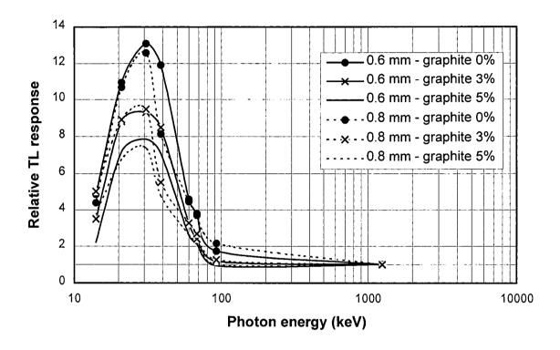
Figure 2: Photon energy relative TL response curve of graphite mixed and pure TL dosimeters with 0.6 and 0.8 mm thick (40 and 50 mg respectively).
