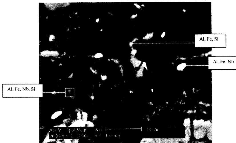
Fig.2- EDS analysis showing distribution of Al, Fe, Nb and Si in the extruded material.
