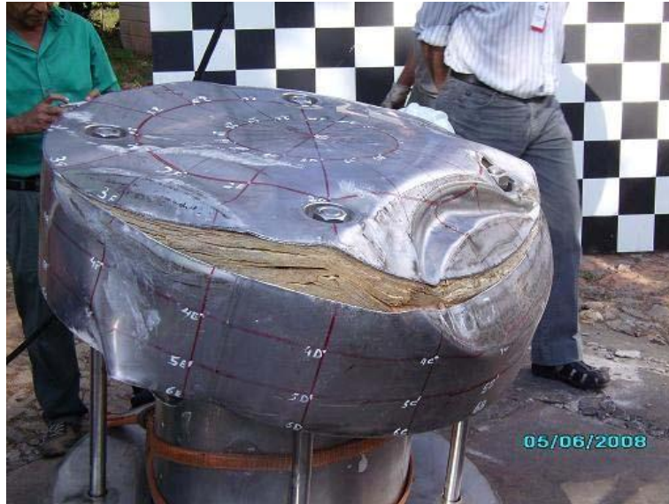
Figure 3. Top shock absorber after the CG-corner 9 m drop test
