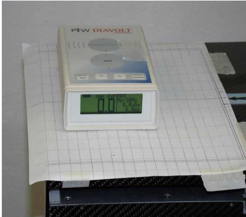
Figure 2. PPV meter on the support.
