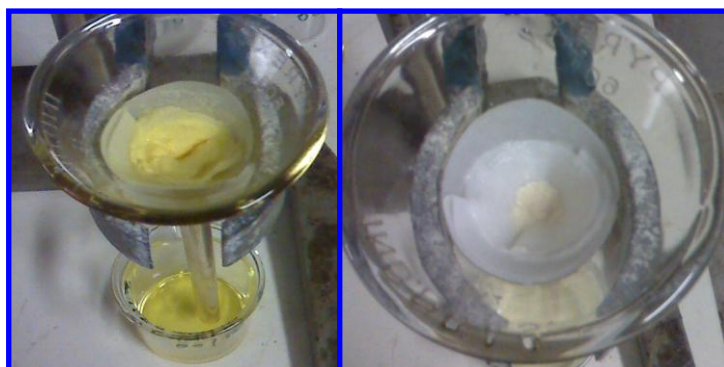
Figure 2. Filtration step of the precipitate of Mo with alpha-benzoin oxime in the presence of U(VI) ions and the washing step of the same precipitate, respectively.
