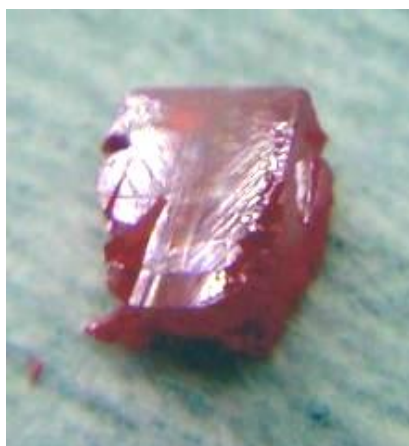
Figure 4 – \text{HgI}_2 crystal grown by PVT technique
