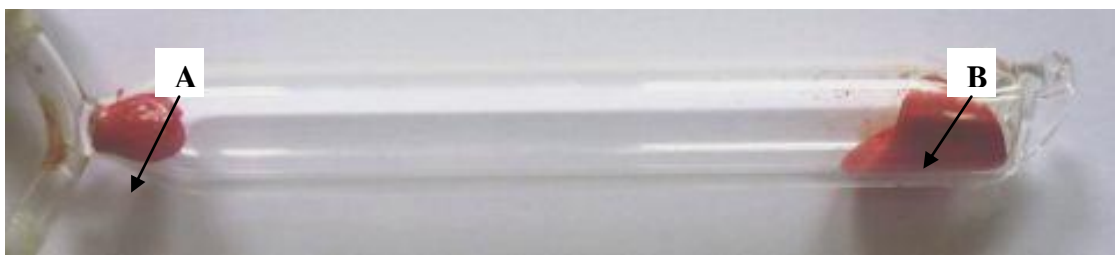
Figure 3 – Sealed ampoule with an \text{HgI}_2 grown (seed) in one of the extremities (A) and the \text{HgI}_2 in another extremity (B)
