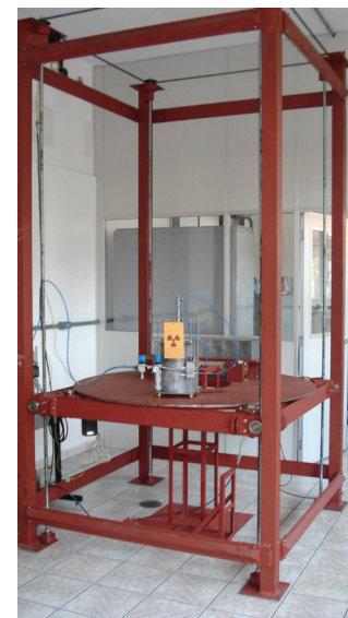
Fig 2- Typical 3th generation CT used in lab for industrial objects design optimization.
