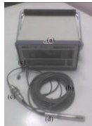
Fig. 1 Example of dosimeter clinical: (a) electrometer. (b) Cables. (c) connectors.(d) ionization chamber
