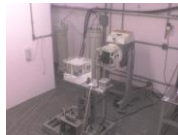
Fig. 2 Irradiation Room consists a Gamatron radiator system of Co-60, acrylic phantom with distilled water and holder's, thermometers, air conditioning, humidifier, hygrometer and a table for support
