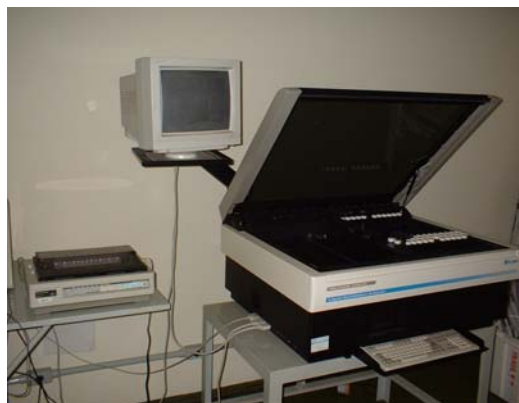
Liquid scintillation counter for Tritium measurement in samples
