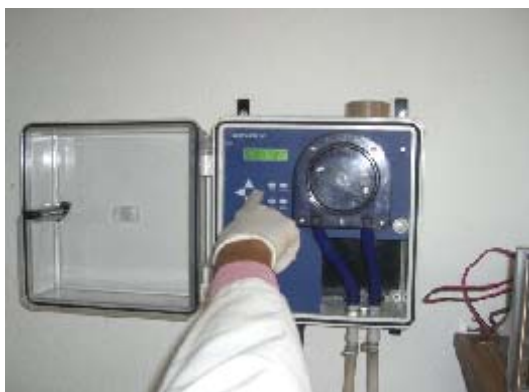
Adjustment of the sampling peristaltic pump in sewerage collecting sample
