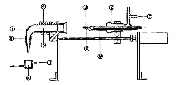
FIG.1 - Schematic diagram of remotely controlled automated apparatus for dry distillation of radioiodine from irradiated TeO<sub>2</sub> target: 1. Outer quartz tube (fixed). 2. Inner quartz tube (movable). 3. Platinum support with TeO<sub>2</sub>. 4. Induction coil. 5. Pt tube  $\neq = 22$ mm. 6. Thermo couple. 7. O<sub>2</sub>flow (30-40ml/min). 8.Heating ribbon. 9. Electrical resistance. 10. NaOH solution. 11. Cooling liquid circulation.
