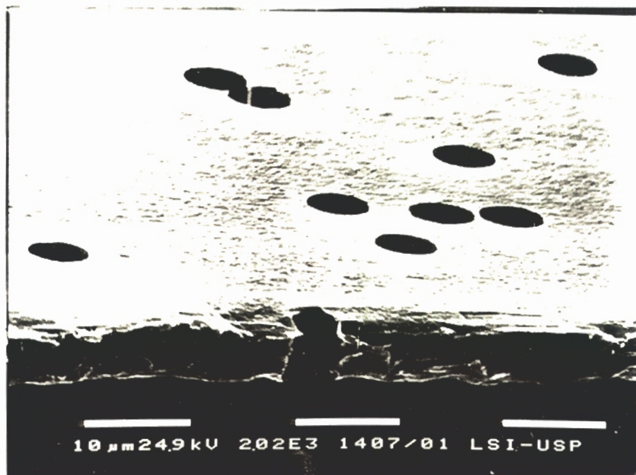
FIGURE 6 Pore size: 5.5 \mu\text{m} . Pore density: 10^5 pores/cm 2
