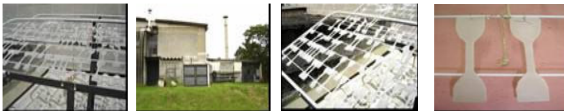
Figure 1. Samples settled in a device for natural ageing assay in the IPEN-CQMA department.
