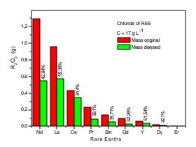
Figure 2 – Fractionation of rare earths in pH 1, with stirring, using Ionac MC-3470XL membrane
