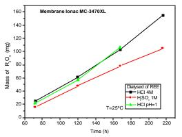
Figure 1 – Behavior of some fractions of rare earths on Ionac membrane dialysis in hydrochloric and sulfuric media
