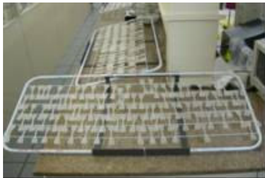
Fig. 1 - Samples settled in a device for assay of natural ageing, confectioned in laboratory.
