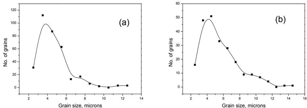
**Figure 2** – Mean grain size distribution for the (a)  $\text{Pr}_{15}\text{Fe}_{\text{bal}}\text{Co}_8\text{B}_7\text{Nb}_{0.05}$  and (b)  $\text{Pr}_{15}\text{Fe}_{\text{bal}}\text{Co}_8\text{B}_7\text{Nb}_{0.05}\text{Ga}_{0.25}$  HD sintered magnets.
