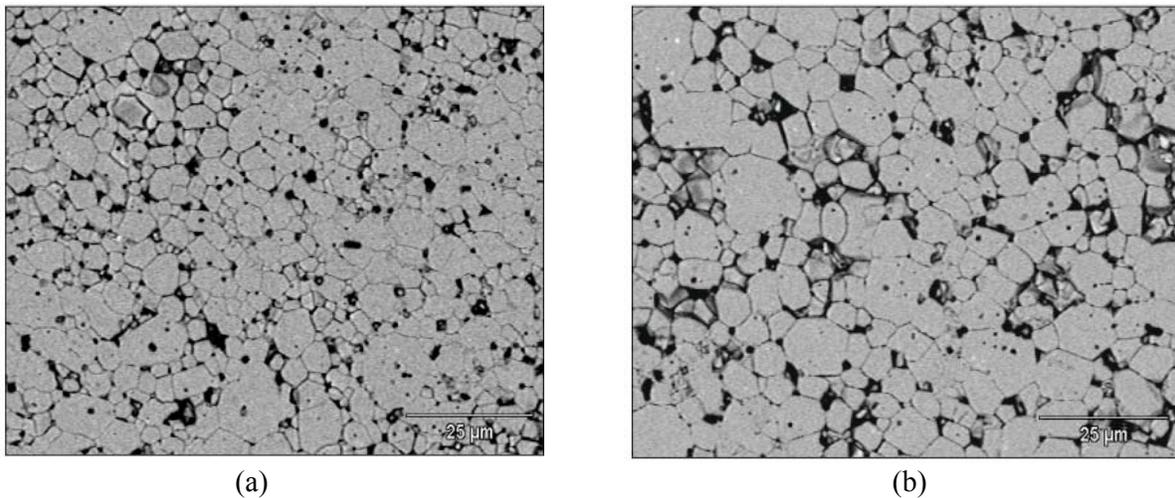
**Figure 1** – Microstructure of the sintered HD  $\text{Pr}_{15}\text{Fe}_{\text{bal}}\text{Co}_8\text{B}_7\text{Nb}_{0.05}$  (a) and  $\text{Pr}_{15}\text{Fe}_{\text{bal}}\text{Co}_8\text{B}_7\text{Nb}_{0.05}\text{Ga}_{0.25}$  (b) magnets (etched surface; magnification: 1000 X).
