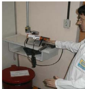
(b) Portable contamination monitor located at the exit of radiological area
