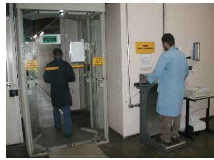
(c) Surface contamination monitor type feet and hands, located in the exit of radiological area.
