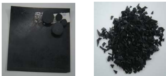
Figure 1 – Model of chloroprene masterbatch obtained from a coil cylinder, before and after cutting.
