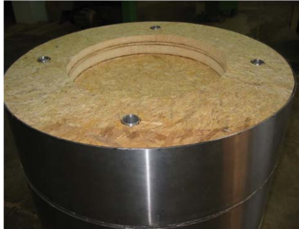
Figure 3- Bottom shock absorber partial assembling.
