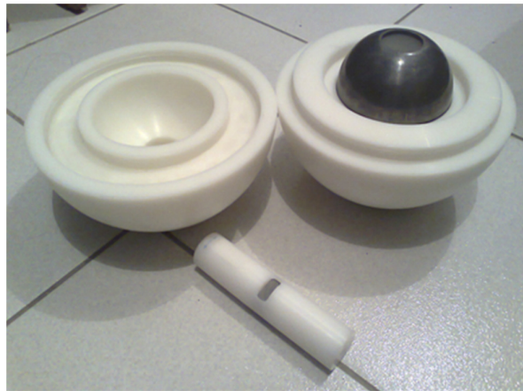
Figure 3. Passive dosimetric system, based on CR39 PADC on polyethylene/lead sphere.
