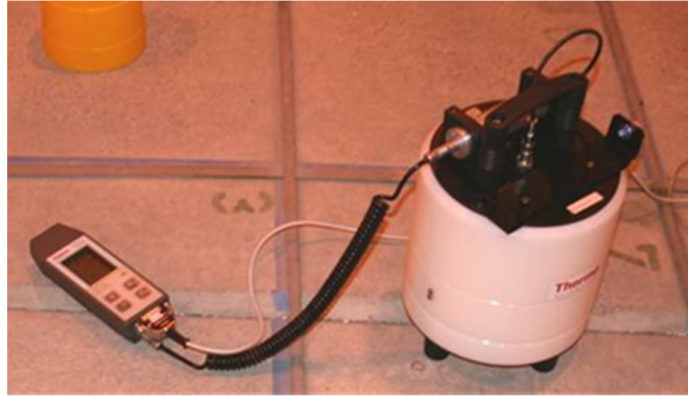
Figure 2. Monitor FH40G-10 with FHT-762 neutron probe [14].
