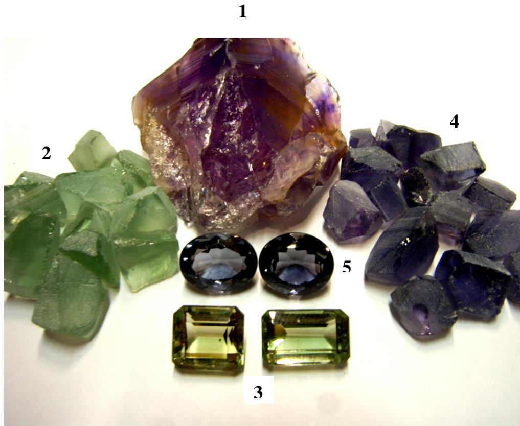
Figure 1. (1) Natural amethyst Montezuma; (2) Prasiolite (burnt amethyst); (3) Prasiolite cut and polished; (4) “Safirita” (burnt amethyst and irradiated); (5) “Safirita” cut and polished.
