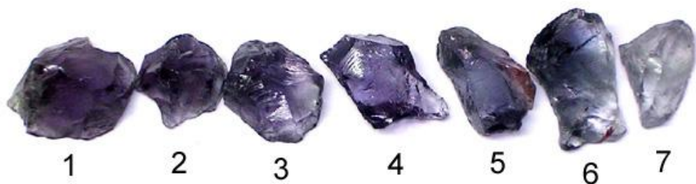
Figure 3. Variations of the shade of blue produced by heating of opaque samples
