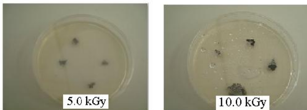
Figure 5. Two days of incubation, sings of fungus activity. Oil irradiated with 5.0 and 10.0 kGy with 50% of concentration.
