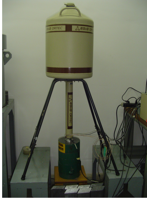
Figure 4. The detection system of hyper-pure germanium (HPGe).
