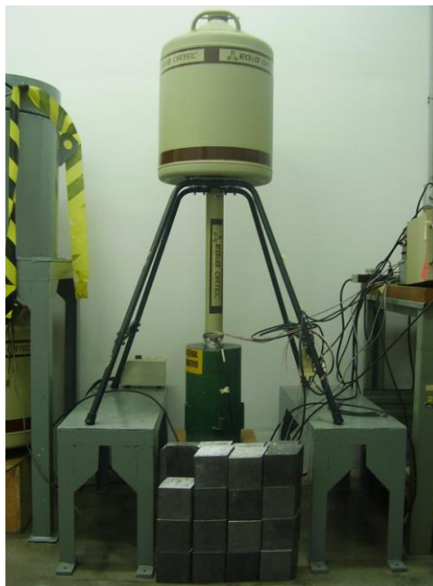
Figure 3. System of high purity Germanium (HPGe) detector.
