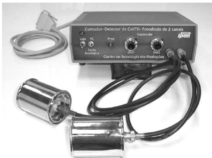
Fig. 3. Picture of the portable counter, constituted of two CsI(Tl)-PIN photodiode detectors, amplification units and signal processing.
