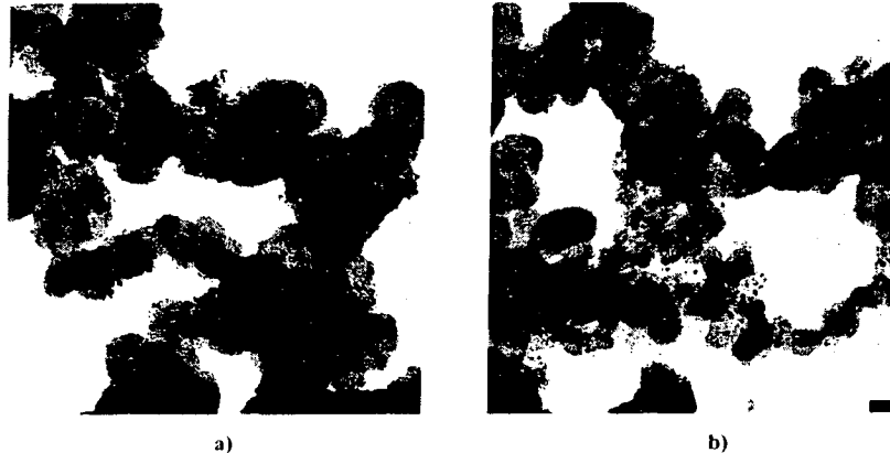
Figure 1: TEM micrographs a) electrocatalyst treated at 400°C under hydrogen flow and b) treated at 400°C under hydrogen flow and submitted to the oxidative thermal treatment.
