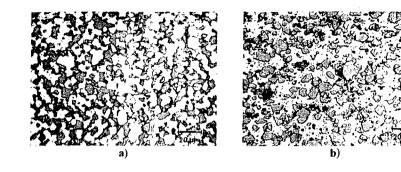
Figure 1. Optical micrographs of the spray formed alloys, where the homogeneity of the silicon particles is observed. a) Alloy 1. b) Alloy 2.
