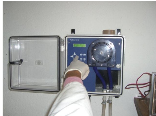
Adjustment of the sampling peristaltic pump
