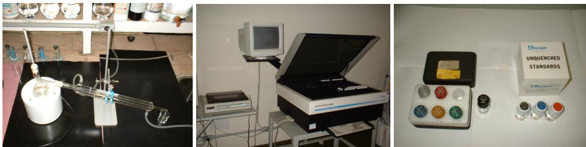
Figure 3. Distillation apparatus, liquid scintillation counter and quenching standard solutions
