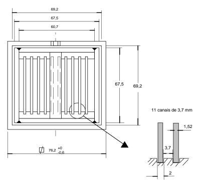
Figure 2. Transversal section of the MID (dimensions in mm).
