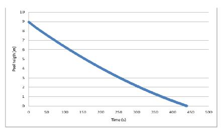
Figura 7. Time to drain the reactor pool down to the level of the bottom of the core during a Primary Coolant Boundary Rupture postulated accident.
