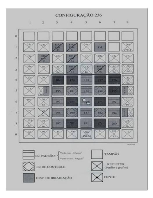
Figura 3. - IEA-R1 reactor core.
