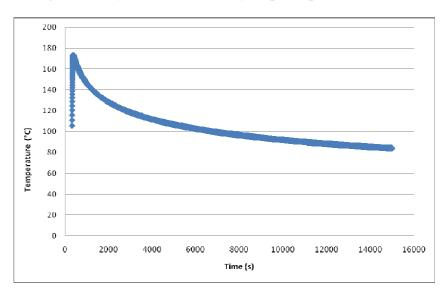
Figura 8. Minplates temperatures achieved after core draining in a postulated Primary Coolant Boundary Rupture accident.
