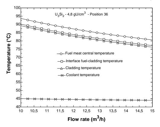
Figura 4. Fuel miniplate and coolant calculated temperatures versus MID coolant flow rate (U<sub>3</sub>Si<sub>2</sub> – 4.8 gU/cm<sup>3</sup> – Position 36 of the matrix plate of IEA-R1 reactor.
