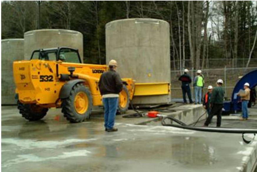
Figure 4. Handling of SNF casks by a lift truck [12]
