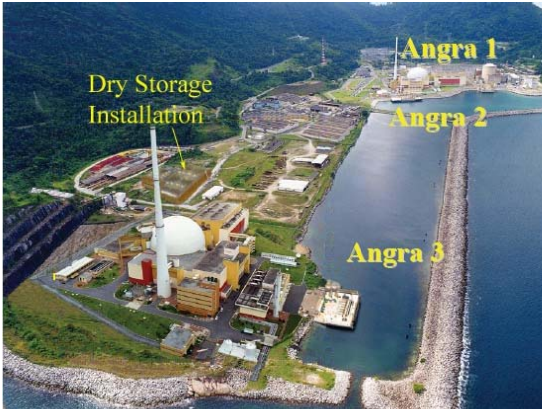
Figure 6. Possible location of the SNF dry storage installation at the Angra's reactors site.
