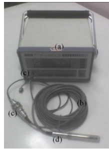
Figure 1: Standard clinical dosimeter of LCI: (a) eletrometer. (b) cable. (c) conector. (d) ionization chamber.
