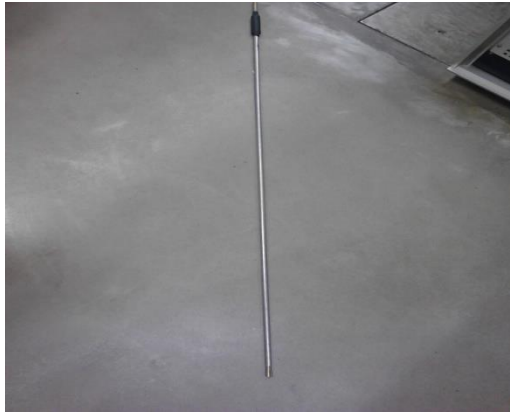
Figure 5 - Tool for removal of fuel rods [7].
