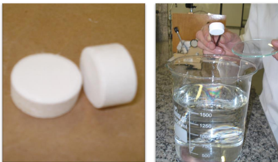
Figure 2: Tablets produced with NaDCC in combination with adjuvant agents
