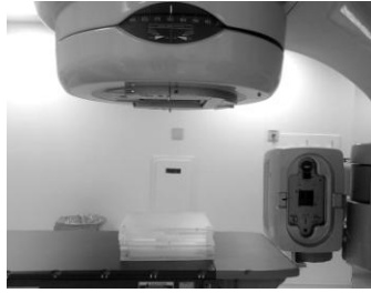
Figure 2: PMMA phantom and TLDs electron beam irradiation set up.
