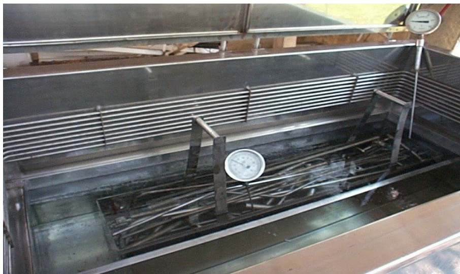
Figure 8: Surface decontamination of surfaces of parts via ultrasound
