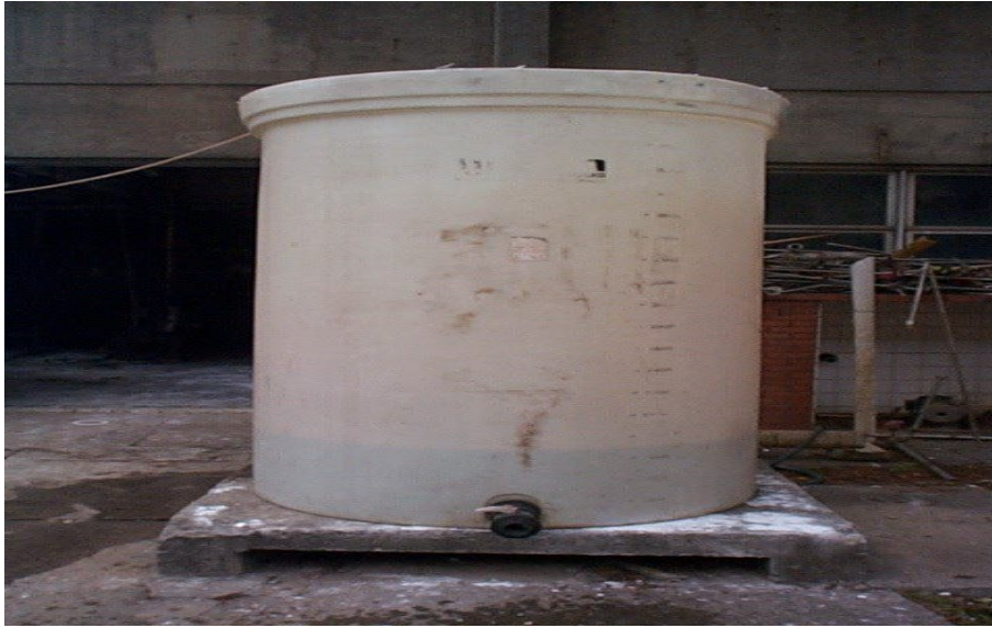
Figure 9: Surface decontamination of surfaces of parts via immersing
