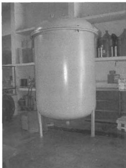
Figure III: CDTN pressure tank for water immersion test
