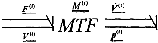
Fig. 1. Modulated ith-component inertial transformer.
