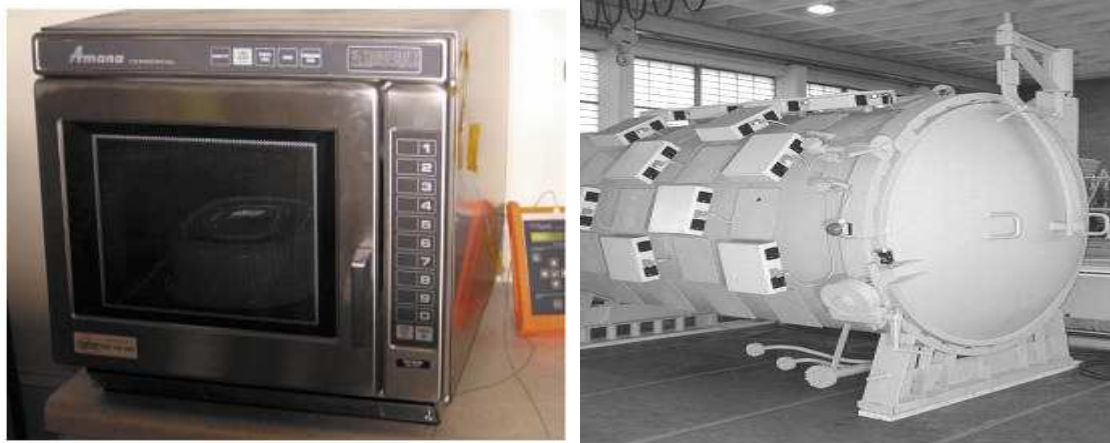
Figure 2: Kind of microwave irradiator, a domestic adapted model [10] and an industrial model [11].
