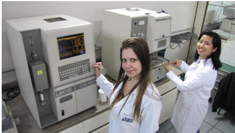
Figure 1: Characterization of Carbon and Sulfur by Radio Frequency gas extraction combustion coupled with Infra-red detector method, LECO CS-400.
