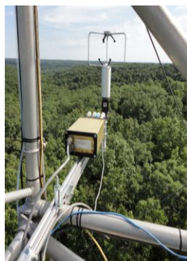
Figure 1: REA system coupled to the sonic anemometer device on the top of the tower.
