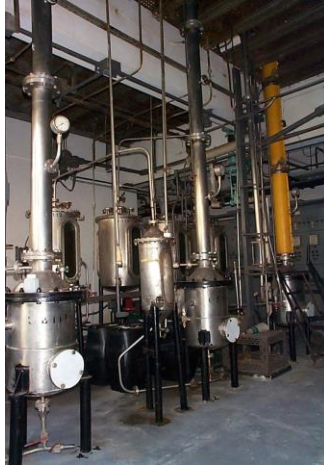
Figure 5: Uranyl nitrate purification pilot plant.
