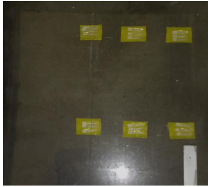
Figure 4 : Assembly of the plaque with TLDS to irradiated inside IPEN/MB-01 reactor
