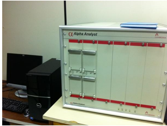
Figure 3: Alpha spectrometer used for the determination of Po-210.
