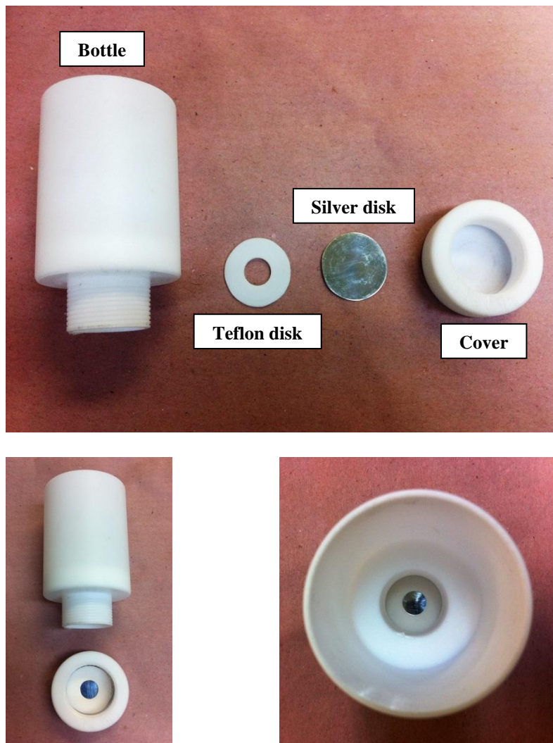
Figure 2: Apparatus used for spontaneous deposition of Po-210.
