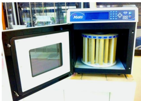
Figure 1: Digestion of the samples in the microwave.
